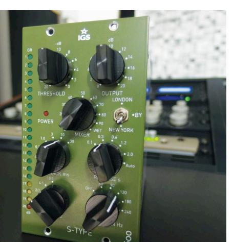
The IGS Audio S-Type 500 is a modern take on the famous SSL Bus Compressor. This is a modern SSL Bus Compressor with better specifications that can be used in more applications, including mastering. New features (e.g., the ability to filter the side chain) add versatility to this compressor.
