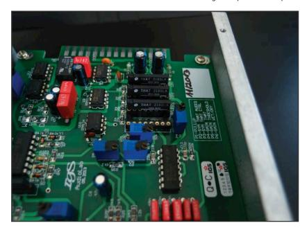
The S-Type 500 uses eight THAT 2180LA ICs instead of the now-unavailable DBX 202XT used in the original SSL Bus Compressor. One of this compressor's notable features is its use of TI/Burr-Brown OPA134 series op-amps, which are more than twice as fast as the NE5532s used in the original model and other SSL clones. OPA134s provide better noise and THD levels, which makes the S-Type 500 a cleaner sounding compressor.
