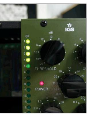
Operating the S-Type 500 is fairly easy. It uses stepped switches on most functions which add a sturdy, quality feel to the unit. The LED gain reduction meter on the compressor's side displays up to 20 dB of gain reduction in 1 dB steps.
